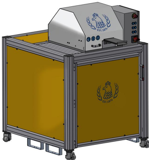
Figure 2: Frame with enclosure and protective devices
